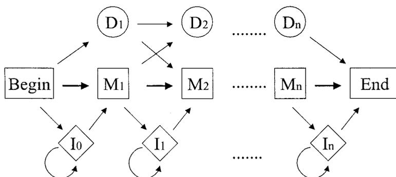
**FIG. 1.** Overview of the plan 7 architecture of HMMER 2.2. D stands for delete state, M for match state, and I for insert state. Arrows indicate the allowed transitions between states.
